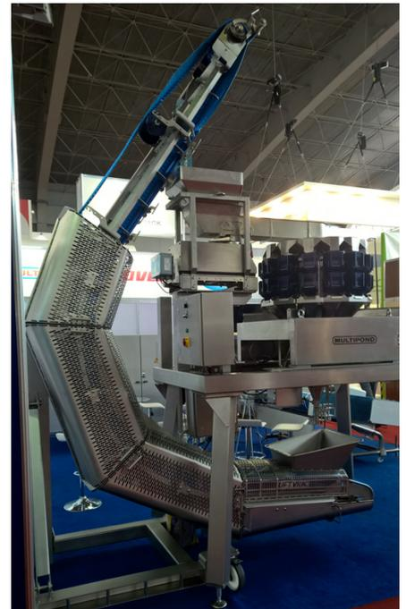
*C-shaped Liftvrac : the space-saving champion (above with a Multipond multihead weigher, herebelow feeding a mixer placed next to a mincer)*
